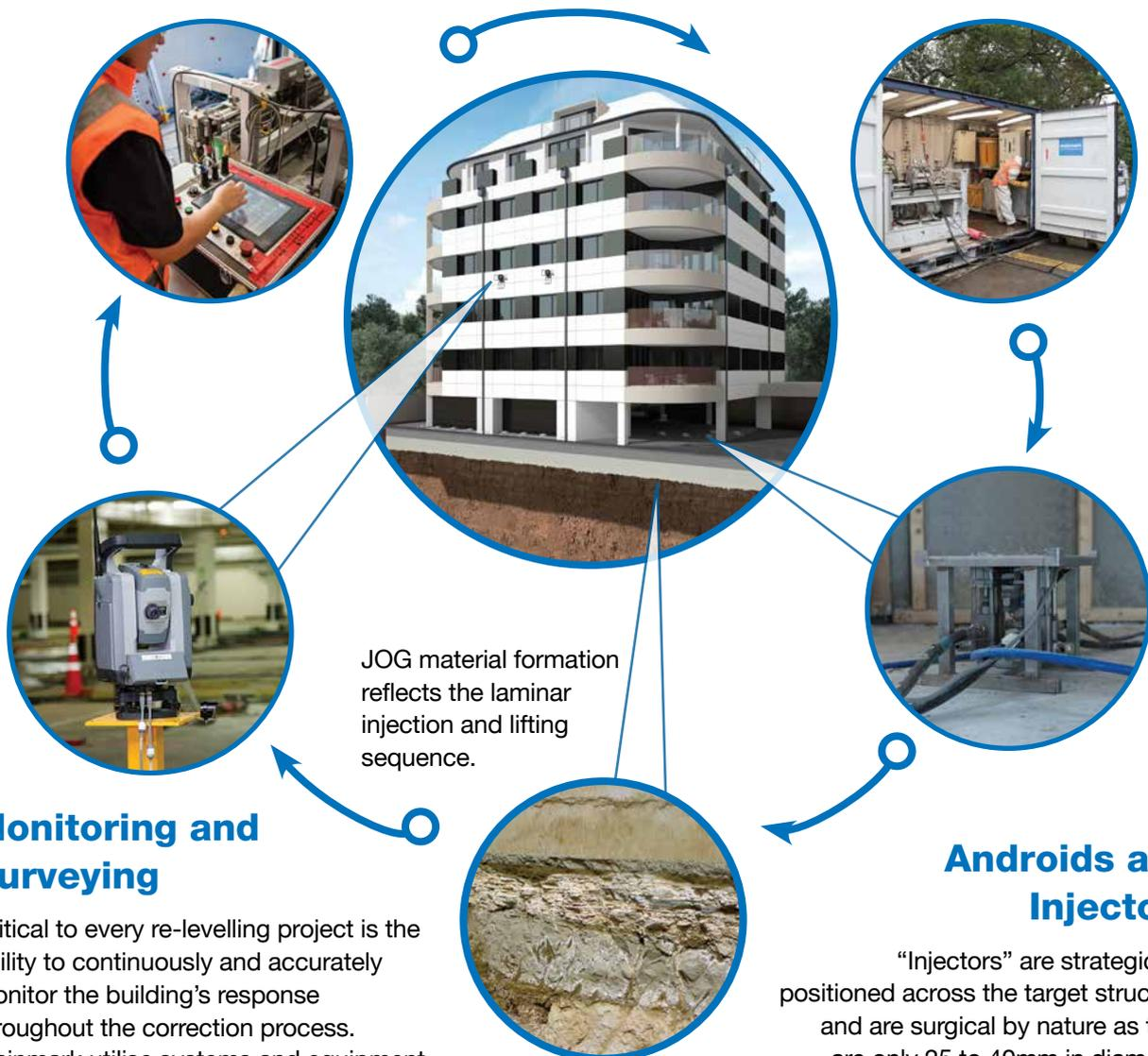
JOG material formation reflects the laminar injection and lifting sequence.
